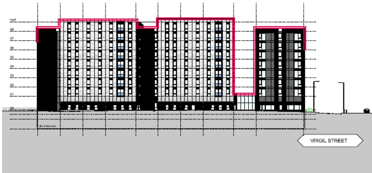
Our detailed technical analysis indicates that 237/237 (100%) of the windows assessed will meet the VSC daylight targets. The BRE suggests a further, more detailed test for daylight can be undertaken known as Average Daylight Factor (ADF). This test considers the room use, as well as other factors such as volume, layout and internal reflectance. The ADF test indicates that 222/222 (100%) of the rooms analysed will meet the ADF targets.
