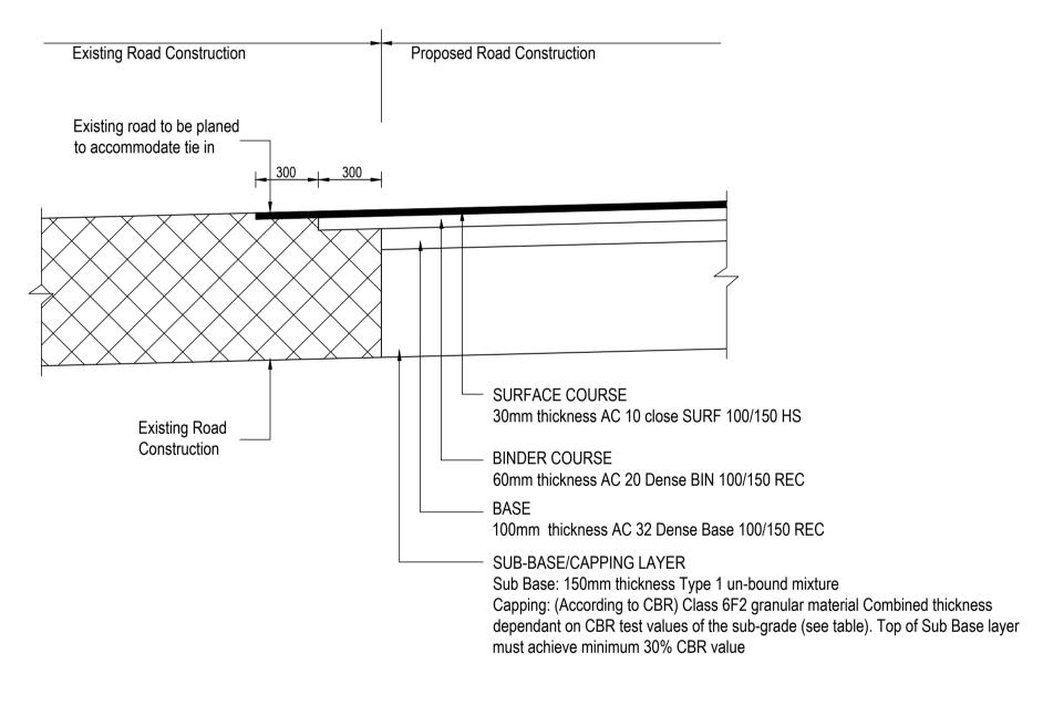
PROPOSED/EXISTING ROAD TIE IN DETAIL SCALE 1:20
